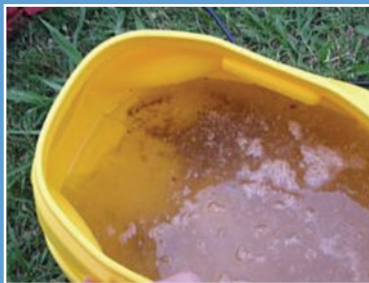
Water from an untreated drain pan
